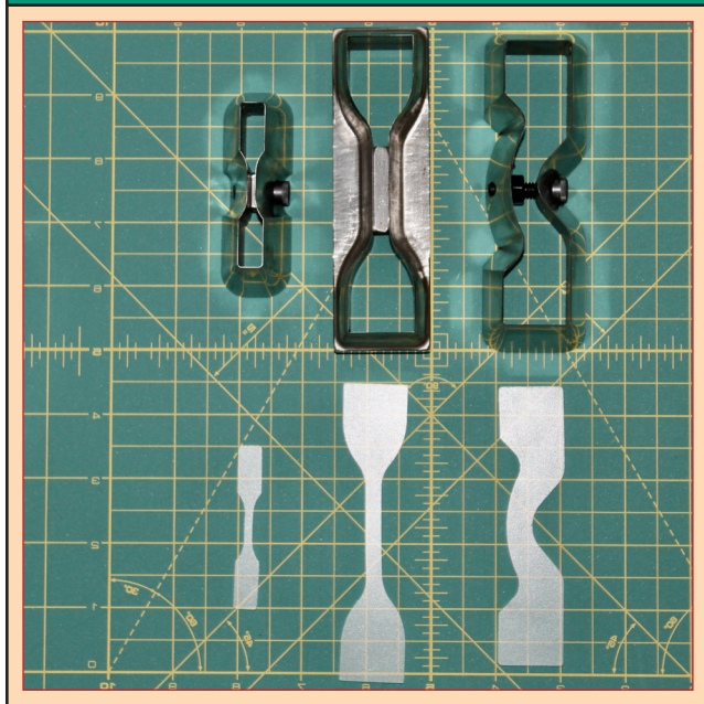
Figure 5 - ASTM Instron dies: D638V (left); D412C (center); D624B (right)
