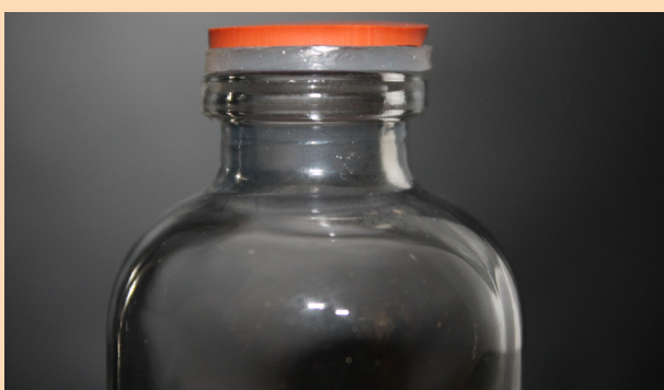
Figure 13 - bilayer ExSil septum structure on modified serum bottle
