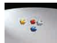
Water droplets on silicon wafer treated with SIH5841.5 exhibit high contact angle
