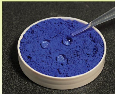
SS treated powders are hydrophobic and resist wetting by water. (Ultramarine Blue SS)
