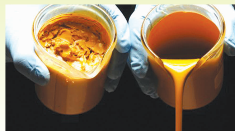
untreated yellow iron oxide in ethylhexylpalmitate
