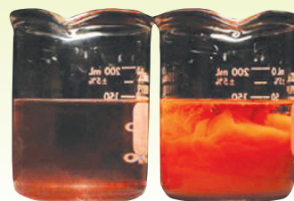
untreated yellow iron oxide in water HS treated yellow iron oxide in water
