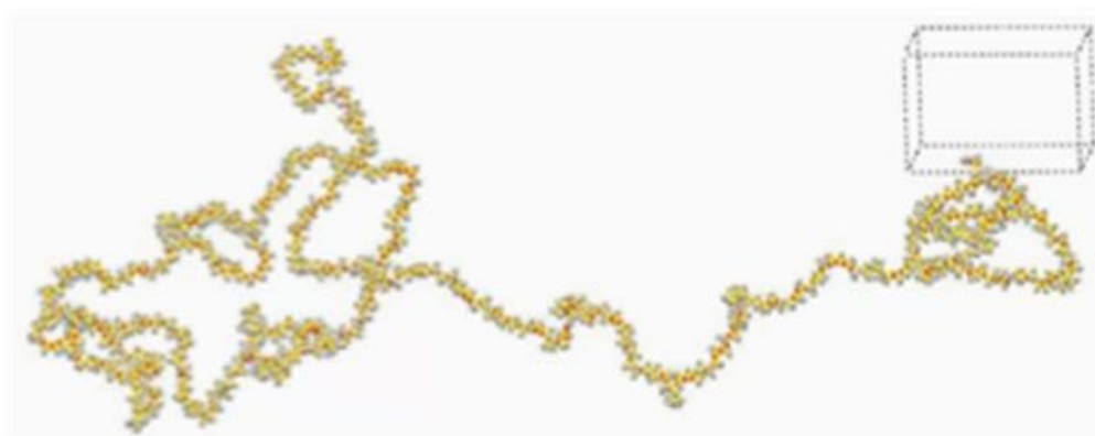
Figure 10. Atomistic model of a 50,000 Da segment of ultra-high elongation elastomer suggesting 1–2 knots. (Author's work).
