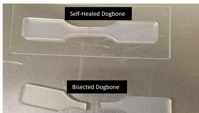
Figure 12. Pseudo-self-healing demonstration of bisected specimen of ExSil® (Author's work).
