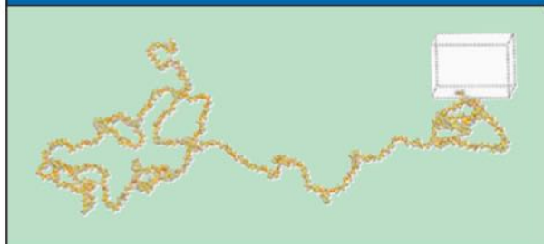
Figure 5 - atomistic model of a 50,000 MW segment of ultra-high elongation elastomer
