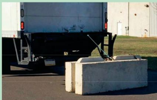
Figure 12 - a solid 1 meter x 9 mm diameter section of ExSil 100 at 0% (12a and 12b) and ~ 2,000% elongation (12c)
