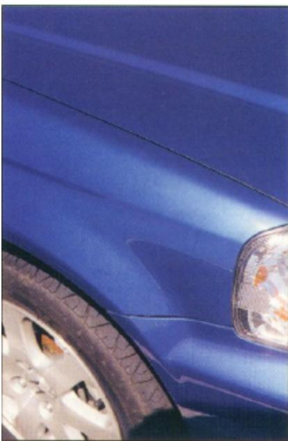
Figure 4. Automotive finishes such as that on the Honda Civic have depth, luster, and environmental resistance that is the result of a complex mixture of hybrid organic-inorganic materials cured into mixed-graft interpenetrating polymer network systems.
