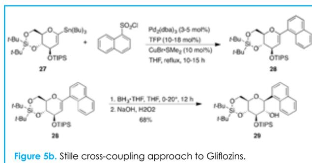
Figure 5b. Stille cross-coupling approach to Gliflozins.
