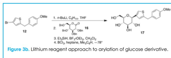
Figure 3b. Lithium reagent approach to arylation of glucose derivative.
