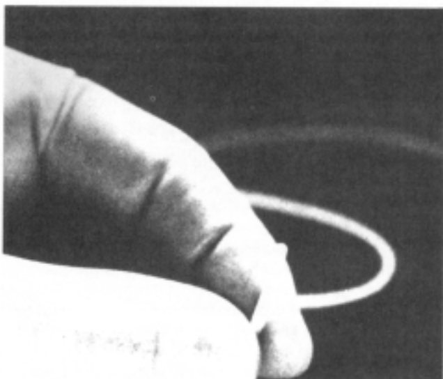
Photo 10. Catheter tubing extruded from Rimplast silicone-urethane and silicone-nylon 12 systems exhibits greater mechanical strength and tear resistance than traditional silicones while maintaining physiological inertness (Petrarch Systems)
