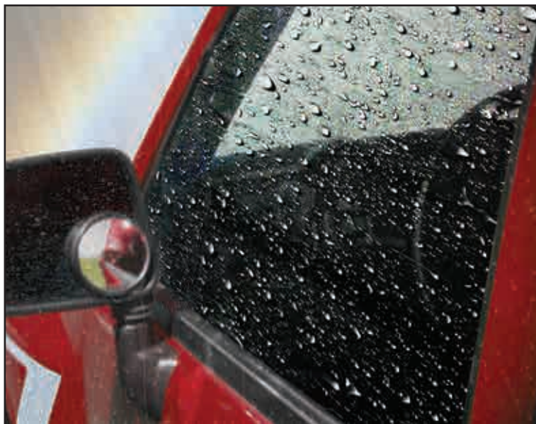
Automotive side windows are treated with fluoroalkylsilanes to provide self-cleaning properties. Water beads remove soil as they are blown over the glass substrate during acceleration.
