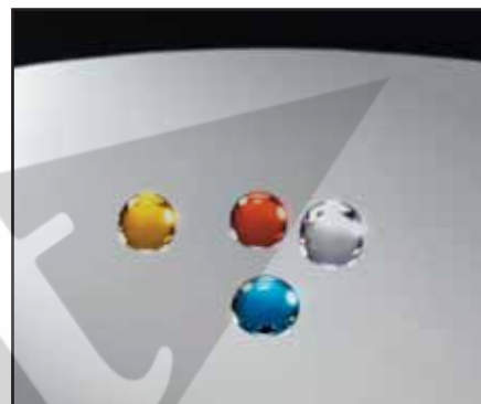
Water droplets on a (heptadecafluoro-1,1,2,2-tetrahydrodecyl)trimethoxysilane-treated silicon wafer exhibit high contact angles, indicative of the low surface energy. Surfaces are both hydrophobic and resist wetting by hydrocarbon oils. (water droplets contain dye for photographic purposes).
